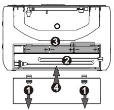
4.) Slide the battery cover upward until it snaps back into place.
